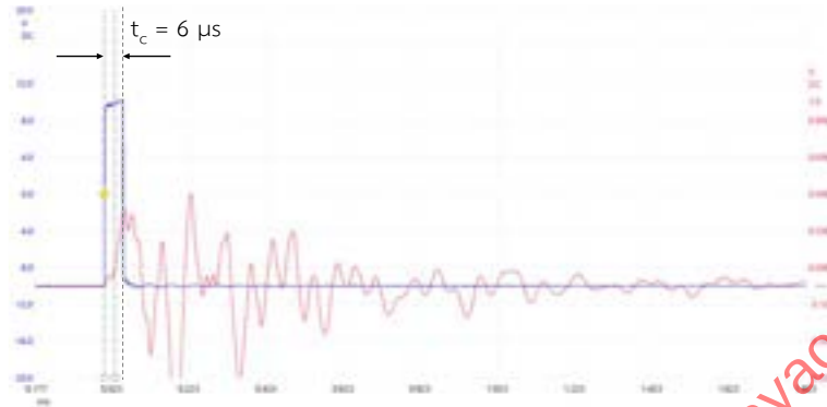
Figure 4-38 Measurement of calibration time for 1 square signal.
